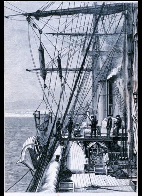
Fig. 17.—The Dredging and Sounding Arrangements on board the 'Challenger.'
